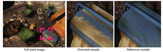
Fig. 7. Example of Z-fighting artifact caused by small precision of the depth buffer.
