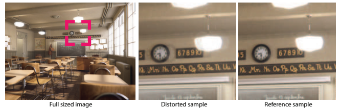
Fig. 11. Example of ghosting as typical artifact of linear warping.
