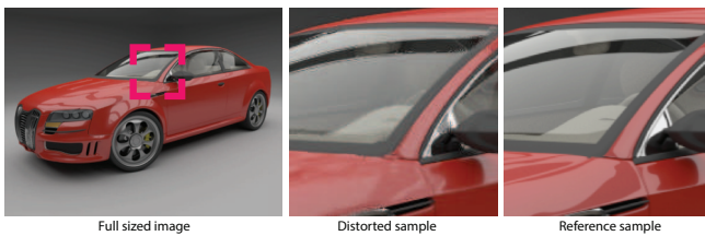
Fig. 10. Double edges and discontinuities caused by optical flow warping method.
