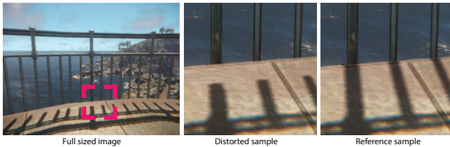
Fig. 5. Example of peter panning artifact - typical 'detached' shadows.
