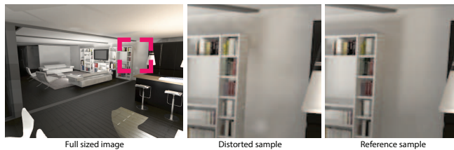
Fig. 1. Example of high frequency noise, common artifact in VPL method.
